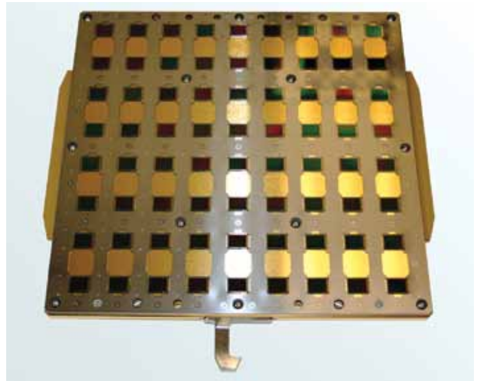
Diced chips fixed on special carrier
