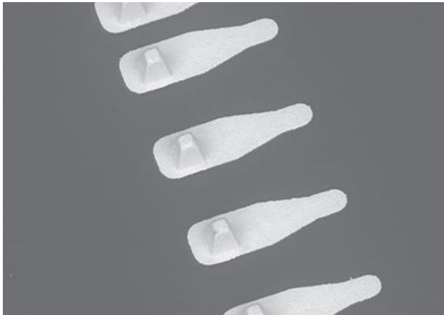
Pyramid Probe tips feature a 12 \mu\text{m} x 12 \mu\text{m} contact area for probing 30 \mu\text{m} x 30 \mu\text{m} aluminum and copper pads.
