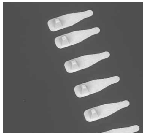
Pyramid Probe tips feature a 12 \mu\text{m} x 12 \mu\text{m} contact area for probing 30 \mu\text{m} x 30 \mu\text{m} aluminum and copper pads.
