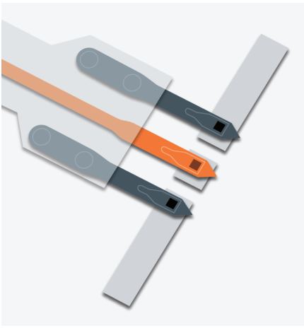
FIG. 3 Example Probe Configuration: GSG on a 101-190C "Open" configuration
