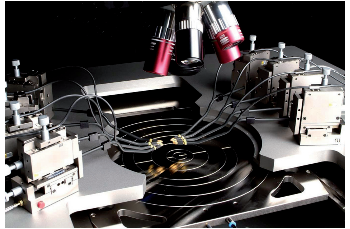
Up to eight positioners can be placed on the PA300DSP.
