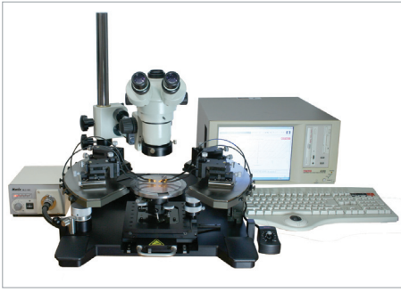
Low-signal option with triaxial measurement capabilities (option: ShieldEnclosure 750 for light-tight, EMI-/RFI-shielded measurements).
