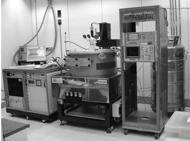
Fig. 1. SUSS PAC200/300 semiautomatic cryogenic probe station
