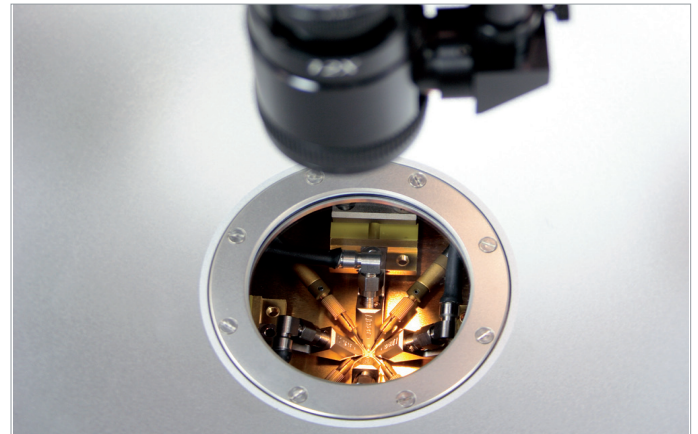
View through the view port of the chamber lid. The shown configuration consists of four RF IZI Probes® and four DC probes.
