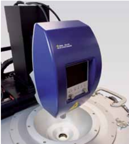
Polytec MSA-500 over topside viewport for mechanical motion analysis
